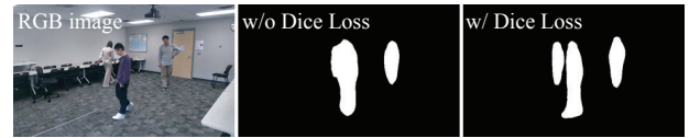
Figure 14: Dice loss improves mask segmentation. Left: RGB image; Middle: results w/o Dice loss; Right: results w/ Dice loss.
